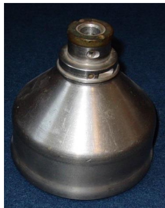
The "separator" bowl Milk entered the hole on top; cream came out the upper outlet and skim milk out the lower outlet (purchased @ Jake Rempel sale)
