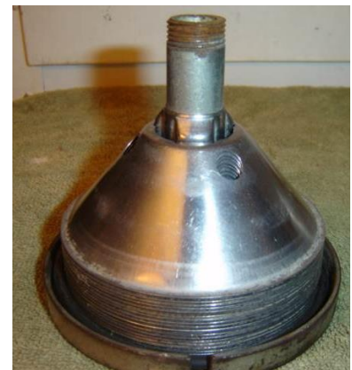
Partially disassembled "separator" bowl showing the stacked conical "skimming disks"
